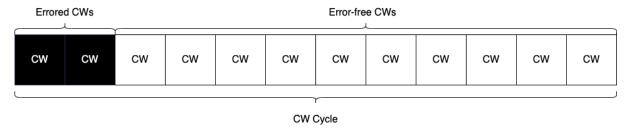
The **Codewords Per Cycle** must be an even integer for 112G serdes, e.g. 2, 4, 6, 8, etc. Inside a cycle, you can configure the number of **Consecutive Errored Codewords**, in which at least one errored symbol is injected:
