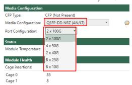
Z800q/Freya-800G-4S-1P G2: Support for 2x40G NRZ TGA - multiple streams with latency and jitter statistics in QSFP-DD cage:
