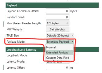
On a stream under the port that has Payload Mode set to Extended Payload, you find the Extended Payload editor as shown below. Click Open Editor and paste the payload data in hex strings and click OK. Then you can see your payload data in a byte-ascii grid view where each row contains 16 bytes.
