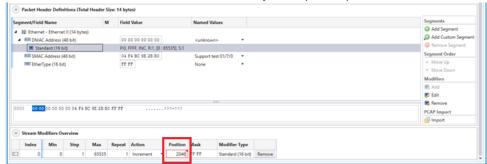
• Odin-10G-1S-6P[b] & Odin-10G-5S-6P-CU[b] – In Segment/Field, for Max Value on 24 bit modifiers the value range has been adjusted to allow valid values.
