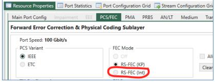
RS-FEC Int (IEEE 802.3ck Clause 161) is supported when the port is configured to 8x100G. To manually set the RS-FEC Int, go to Resource Properties  $\rightarrow$  PCS/FEC  $\rightarrow$  FEC Mode
