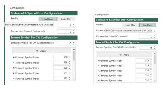
After loading the profile, you can still customize this to meet your test requirements. (Note: you need to click the Apply button to commit the errored symbol index list after loading the profile)
