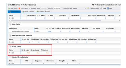
Reconciliation sublayer detection and injection feature (Link Fault Detection/Injection) has been added in ValkyrieManager on the "Layer-1 Control" section on the "Main Port Config" tab for Loki-100G-5S-2P:
