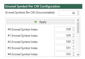
For RS-FEC KP and RS-FEC-Int, a CW with more than 15 errored symbols is uncorrectable, which you can see as you configure.
