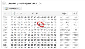
To quickly import the payload data from a pcap file, you can use Wireshark to copy the payload data and then paste it into the Extended Payload editor:
