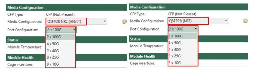
Please note! In QSFP56, QSFP56 (AN/LT), QSFP28 NRZ and QSFP28 NRZ (AN/LT) modes the ports will be split between the QSFP-DD cage and the QSFP112 cage like what was implemented in the QSFP112 modes. Below shows with 2x200G modes on Freya ports = 1 port provided in QSFP-DD cage and 1 port provided in QSFP112 cage:
