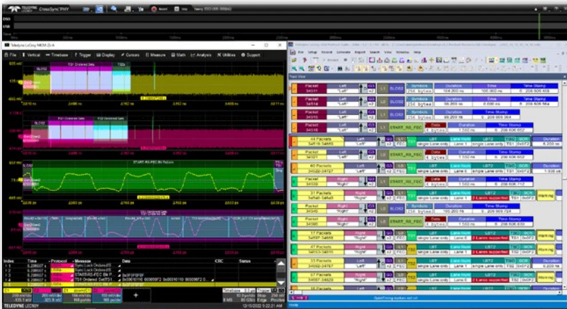
Correlated electrical and protocol views of a link training sequence.
