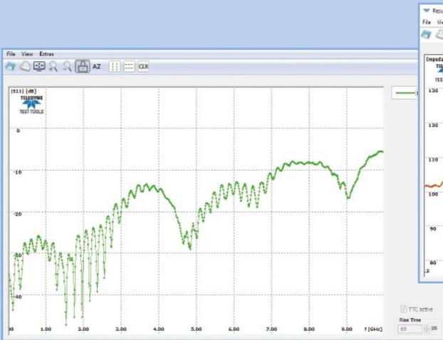
The T3SP15D series offer S-parameter ( $S_{dd11}$  and Full Single-ended, i.e.  $S_{11}$ ,  $S_{21}$ ,  $S_{12}$ ,  $S_{22}$ ) measurements from DC up to 15 GHz
