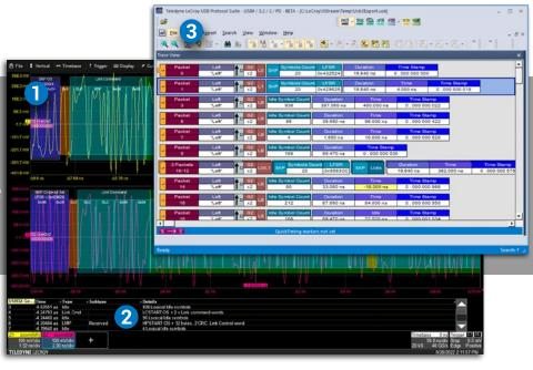
ProtoSync links physical layer waveforms (1), decode annotation and table information (2), and full transaction layer protocol analysis (3). Simply touch a decode table entry in the oscilloscope or a packet in the protocol analysis software and all views are automatically synchronized and aligned. Example shown is USB 3.2 Gen2x2.
