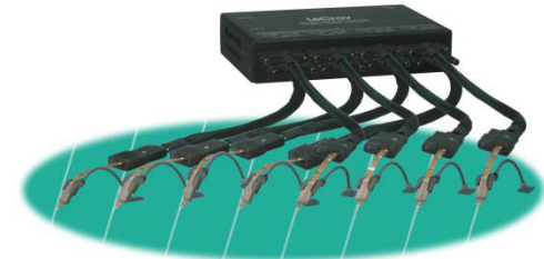
x4 Probe Pod setup, showing support brackets (included in Probe Sets) that assist in holding probe tips in place.
