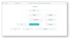
See the LTSSM diagram and check to see how far the device progresses through the initialization setup.
