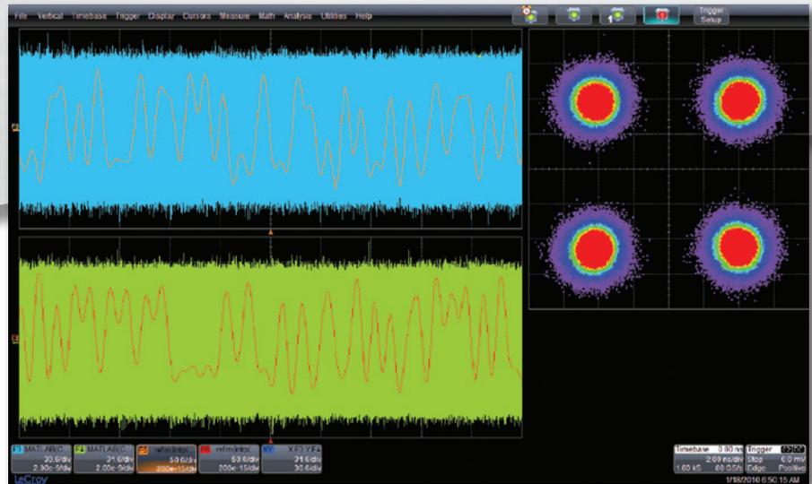
56 Gb/s IQ modulation analysis using the Zi-8CH-SYNCH. In this example, F1 is the math differential result of the optical I+ and I-, and F2 is the differential result of the optical Q+ and Q-. Both signals have been further in-scope processed with MATLAB® (using the LeCroy XDEV option) to simulate receiver equalization.
