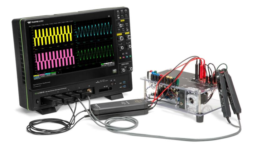
HDO6000B 12-bit oscilloscopes deliver 4 analog channels, 3-phase power analysis software, and high performance probes for inverter subsection, power system and control testing.
