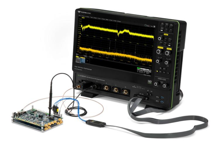
HDO6000B 12-bit oscilloscopes acquire long records at the highest resolution for the most comprehensive deeply embedded computing system analysis (analog, digital, serial data, and sensor).
