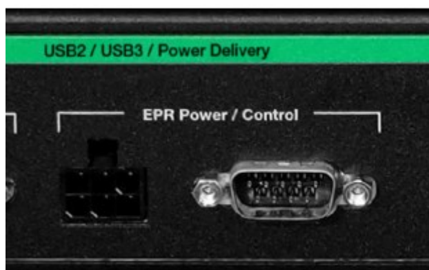
Figure 1: EPR Power / Control connectors
