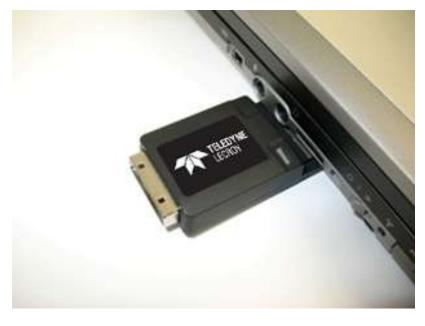
3. Attach the cable by first pulling on the retractor ring which releases the locking mechanism. Connection ends are interchangeable and allow for upstream and downstream transfers.
