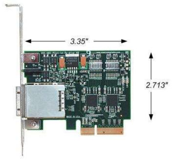
LSIB-HOSTBOARD comes with a bracket for proper 4x motherboard installation.
