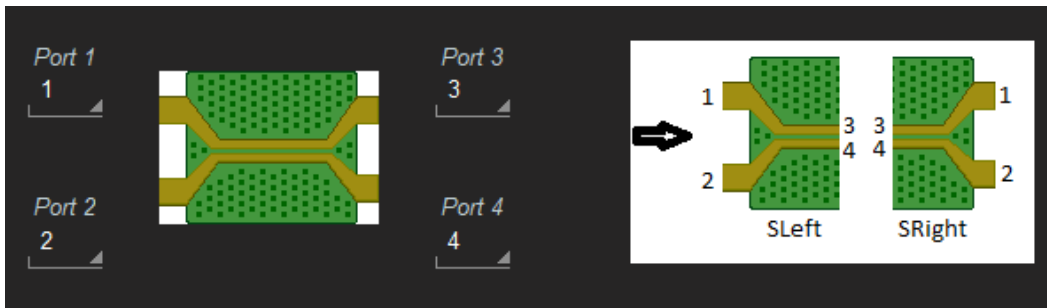
Figure 9: 2X Thru dialog schematic for 4-port S-parameters
