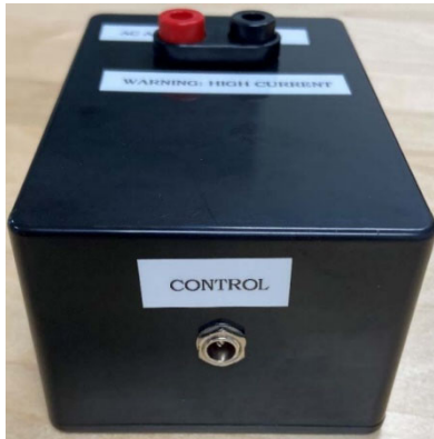
Figure 2: PD Fast Role Swap DC switch Fixture (Note: Available directly from the USB-IF; users must provide their own AC/DC adapter in which the DC side power line is spliced and connected to the +/- power jacks)
