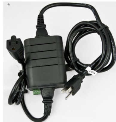
Figure 3: PD Fast Role Swap AC switch Fixture (Note: Available directly from Teldeyne LeCroy; Fixture includes 110V power cords only)
