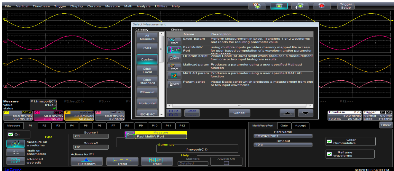
Figure 2: The measure setup showing the FastMultiWavePort setup.
