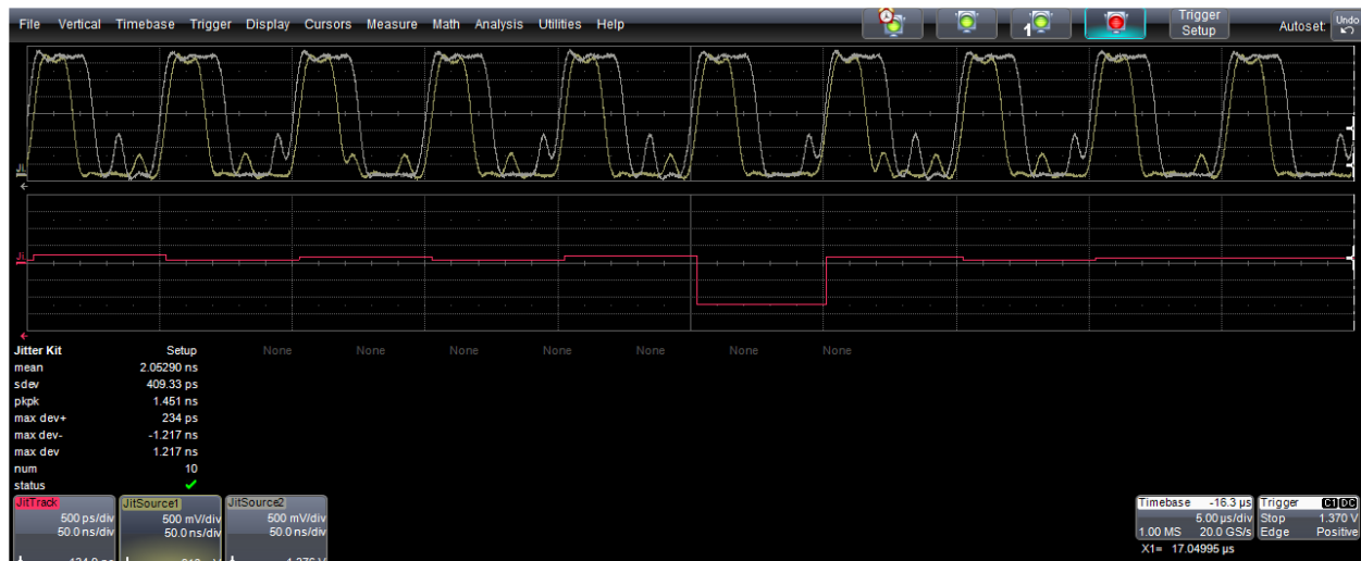
Figure 5: At this point you can see the clock/data pair with the low setup time value
