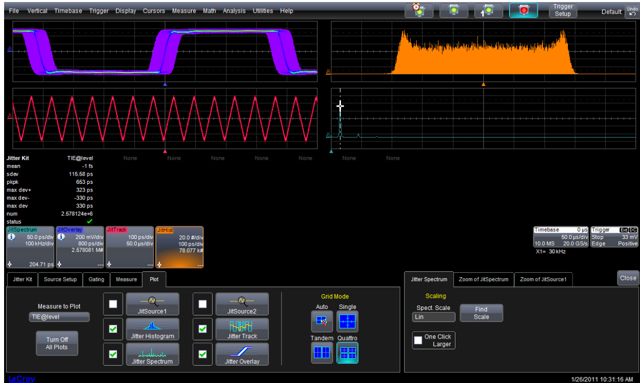
Figure 2: The four Jitter Kit views for a spread spectrum clock and the Plot setup dialog box
