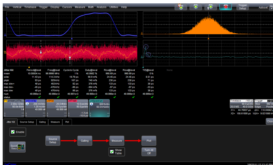
Figure 1: Jitter Kit analysis of a 100 MHz clock signal including jitter measurements and views of jitter in the time, frequency, and statistical domains plus the jitter overlay
