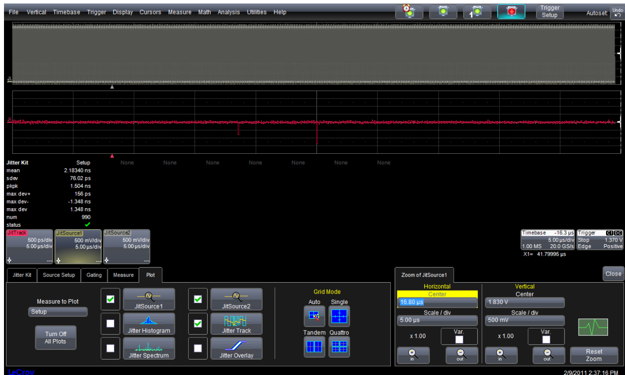
Figure 3: Viewing the input clock and data sources for the setup time measurement along with the JitterTrace of Setup time
