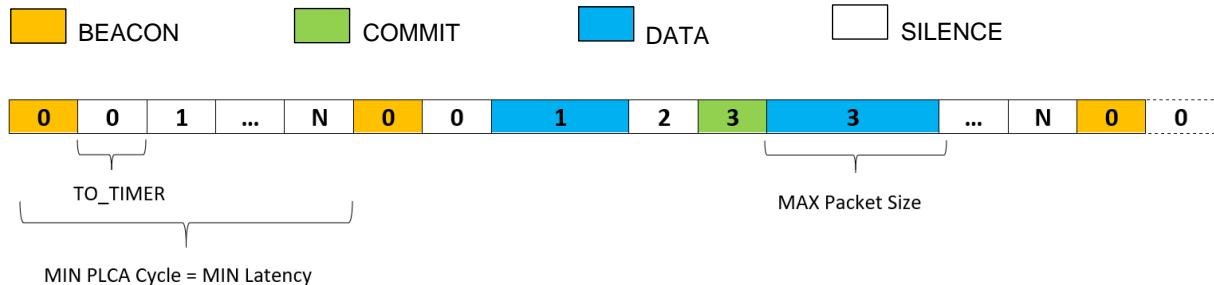
*Minimum latency PLCA cycles. No one has anything to transmit in cycle 1, so total latency is equal only to the number of nodes times the TO\_TIMER. Only Nodes 1 and 3 have transmissions in cycle 2, so all the other nodes cede their transmit opportunity. Node 1 immediately transmits DATA; Node 3 sends a COMMIT followed by DATA.*
