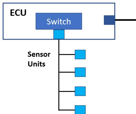
10Base-T1S multidrop topology requires less wire and fewer connectors than legacy topologies.
