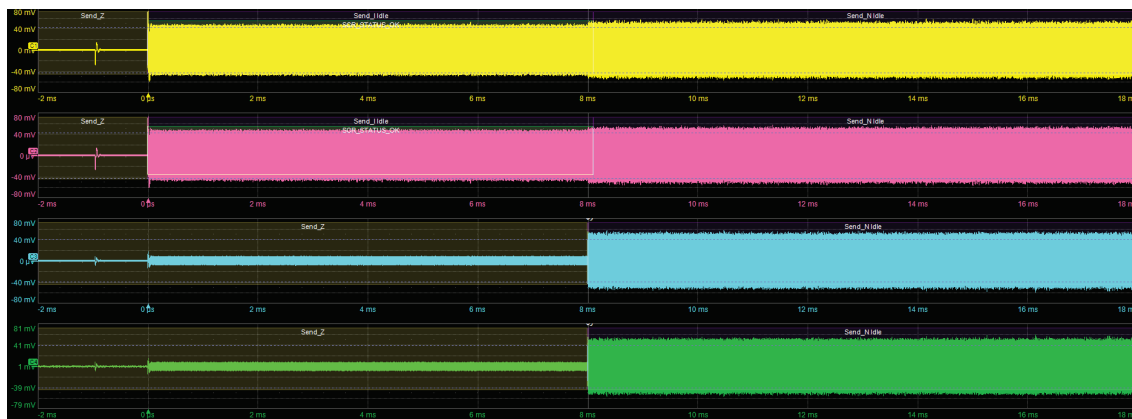
100Base-T1 link startup showing Master (yellow, pink) and Slave (blue, green) switching from SEND_Z to SEND_I and SEND_N.
