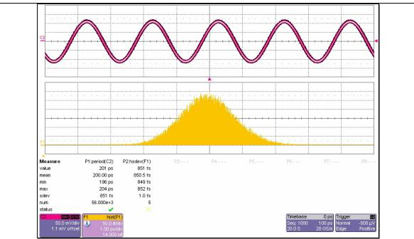
Here is the correct way to measure the period variations. Since the scope is operating in 20 GS/s, it is highly oversampled and SinX interpolation is valid. The correctly measured variation in the period is 851 fs rms.
