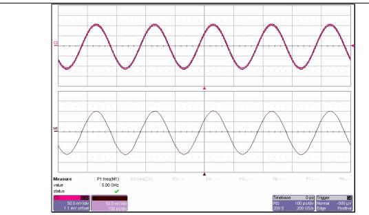
This is a frequency measurement of a sinewave. Note that the sinewave is repetitive and triggered properly. The measurement measures properly the 5 GHz frequency. *Note that not all scopes are even capable of triggering on this signal!*
