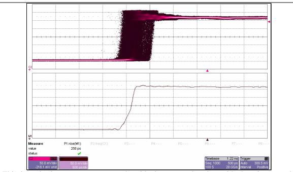
This is a risetime measurement made with the same edge, but with the trigger made purposely unstable. This is not a good use of RIS. Notice that the resulting RIS trace is a smeared version of the multiple traces overlaid.
