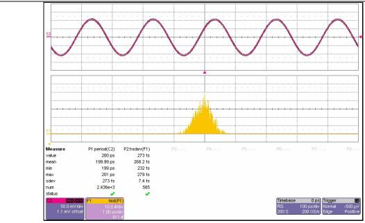
Here is an example of an invalid measurement. The standard deviation of the period is measured as 273 fs - but the waveform is acquired in RIS! Despite the fact that the waveform appears repetitive and a stable trigger is generated, the jitter is a measurement of waveform variations! Since RIS hides any non-repetitive nature of the signal, it should certainly not be used to measure variations in a waveform. It is extremely important to remember this fact.
