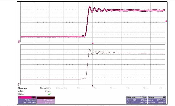
This is a risetime measurement on a fast edge. This is a good application of RIS because the waveform is repetitive and the trigger is stable. Notice that the RIS trace is a clean, noise-free rendition of the input stimulus. The risetime measured is 81 ps.
