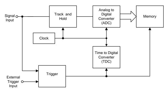
On a WaveMaster, the inter-sample time is 100 ps at 10 GS/s and the discharge time is approximately 5 us max for a trigger that occurs just after a sample is taken. The time is measured with an approximate clock rate of 100 MHz for sub-picosecond resolution.
