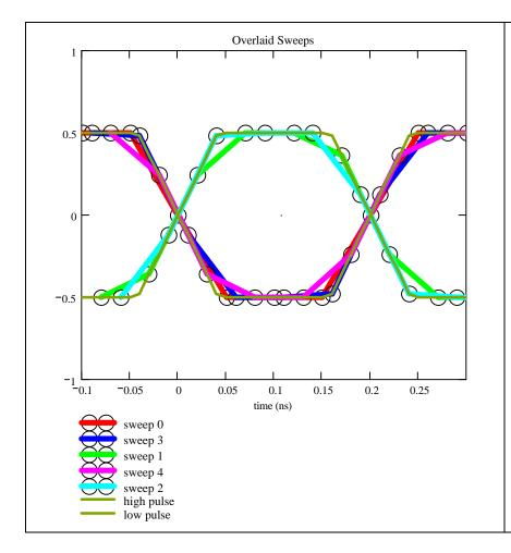
When these sweeps are overlaid, you can see that they form sweeps that overlay the eye pattern. This is what you would see if you repeatedly triggered the scope in single-shot mode. You would observe that this waveform is clearly not repetitive and would not use RIS mode.
