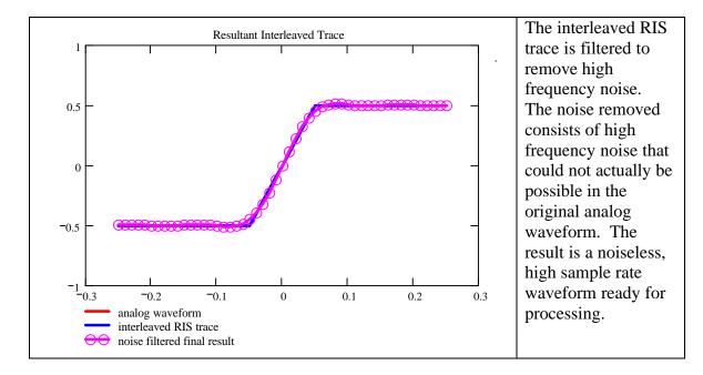
This is how a RIS acquisition should proceed. When used correctly, a very useful waveform is created that can be viewed, analyzed and processed using LeCroy's highly useful waveform processing functions.
