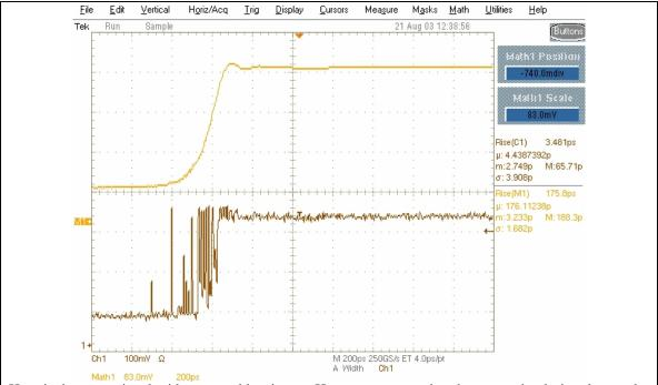
Here is the same signal with an unstable trigger. Here you can see that the scope simply interleaves the multiple waveform segments. The measurement results are, of course, completely useless. When averaging is turned on, you get the same smeared edge as with the LeCroy implementation.
