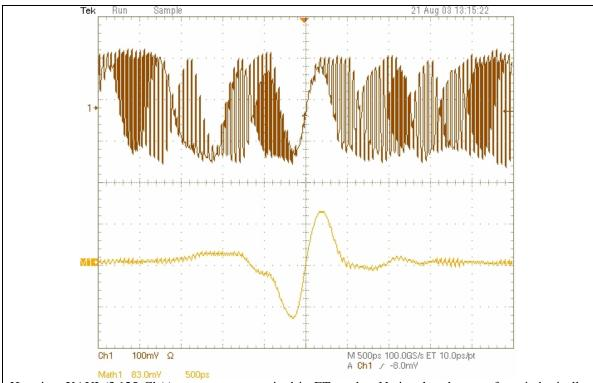
Here is a XAUI (3.125 Gb/s) eye-pattern acquired in ET mode. Notice that the waveform is basically smooth in the region where the bit pattern is repeatable about the trigger. In the region that is not repetitive, meaningless garbage is shown. The averaged waveform shows similar performance as the LeCroy implementation.
