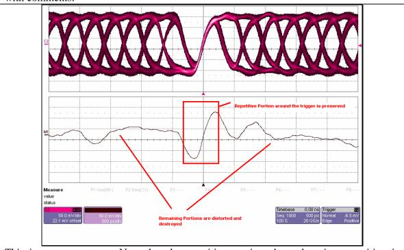
This is an eye-pattern. Note that the repetitive portion about the trigger position is preserved while the non-repetitive portion is destroyed. This is not a good use of RIS because the waveform is not repetitive, as can be seen from the persistence plot.
