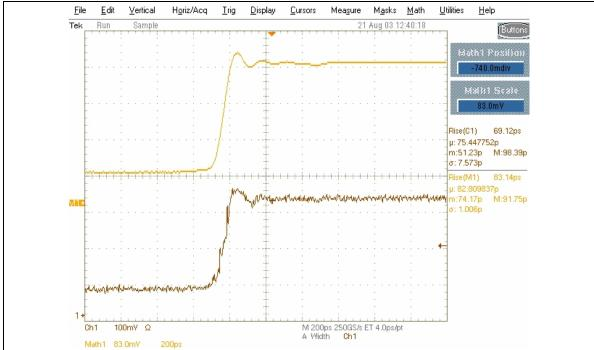
Tektronix 6604 in Equivalent Time (ET) mode. Notice that the trace is noisy and measures risetime with a standard deviation of 7 ps. Averaging is required to get an accurate measurement of the risetime which is 83 ps.
