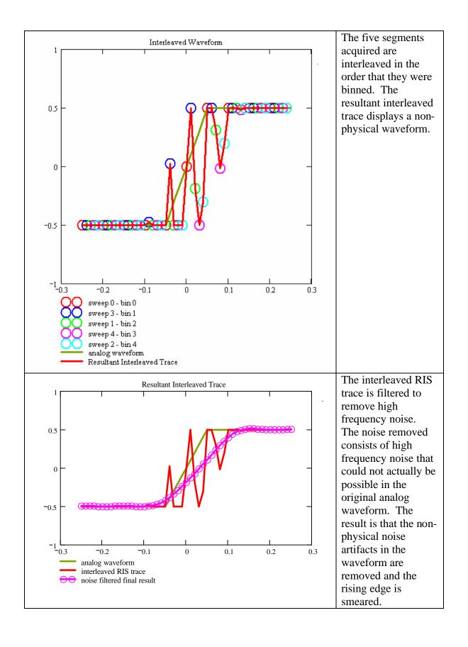
This example demonstrated the effect of an unstable trigger. The resultant waveform is a noise-free, artifact-free rendition of the analog waveform, but the rising edge is smeared. The resulting waveform is severely distorted and not useful. One might conclude from this that since the risetime is reduced, the RIS bandwidth is reduced. This would be an incorrect conclusion since the lower risetime results only from the non-repetitive nature of the waveform.
