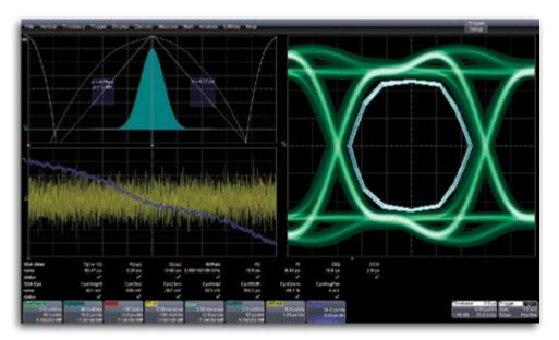
Advanced jitter decomposition methodologies and tools provide more information about root cause. Tj Analysis, RjBUj Analysis and DDj Analysis are made simple with the deepest toolset dedicated to providing the highest level of insight into your serial data signals.
