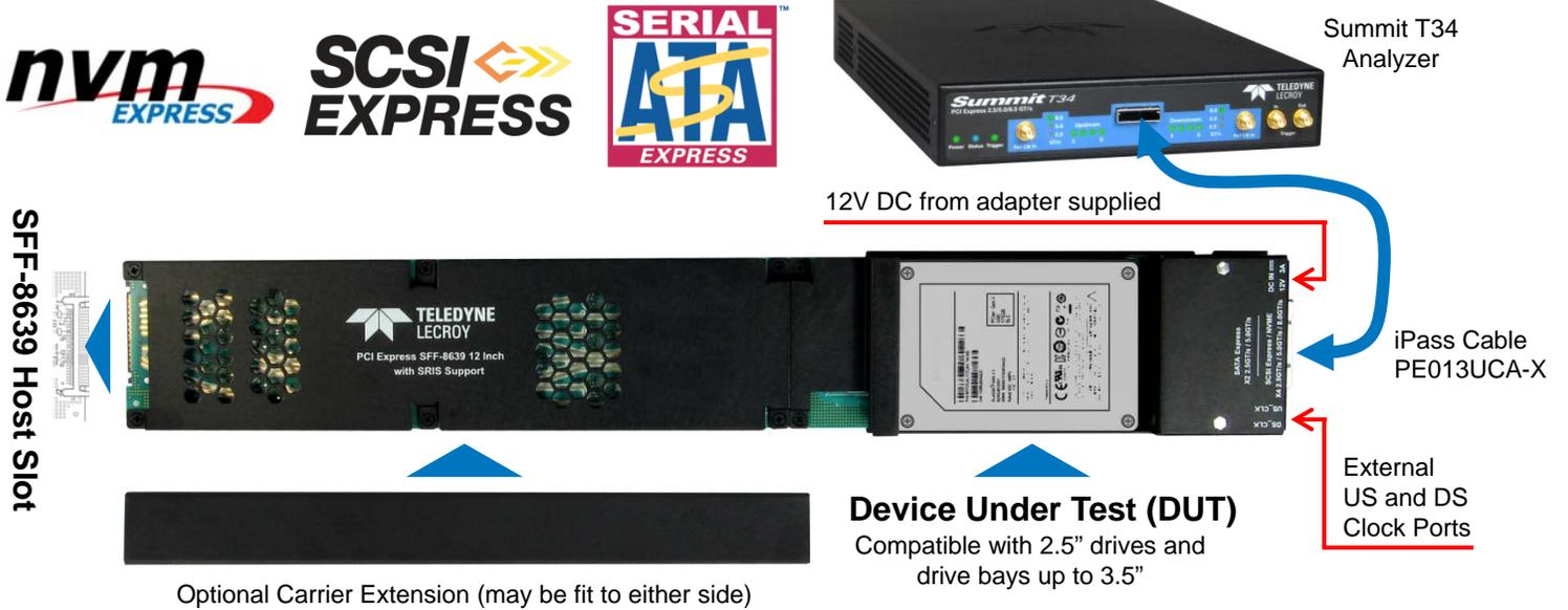
Note: The optional carrier extension(s) can be used to help fit the interposer to a specific manufacturer's drive carrier. This may involve custom modifications to a carrier to allow the interposer to extend out from the end of the carrier. Guidance is provided and an example modification is described in the Quick Start Guide provided with the interposer.
