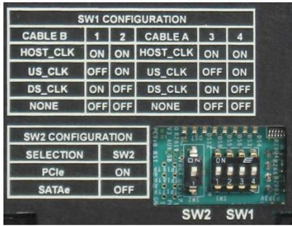
Note: DIP switches and tables shown above are located on the rear side of the interposer
