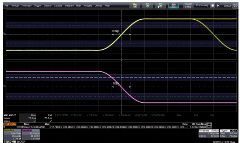
M-PHY measurements are made automatically and compared to the limits in the specification to assess conformance.
