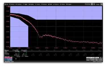
**Transmitter PSD & Peak Differential Output** — The Power Spectrum Density (PSD) of the transmitter is tested against the specified limits defined by the mask while the DUT is transmitting Test Mode 5. Using the oscilloscope for the PSD test removes the need to purchase a spectrum analyzer. The Test Mode 5 waveform is also used to test the Peak Differential Output.
