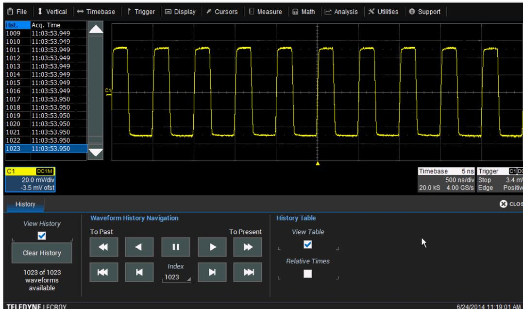
**Figure 2:** Upon invoking the History Mode option by pressing the front-panel button, users are presented with the controls dialog at the bottom of the screen. Checking both View History and View Table brings up the History Mode table seen at top left. History Mode saves and shows all acquisitions automatically with the time at which they were acquired.
