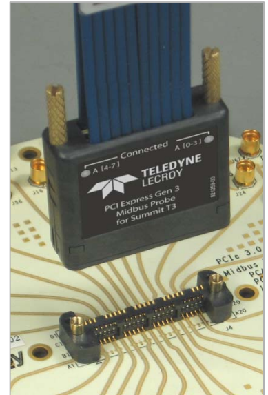
Mid-bus probe provides quick, easy and secure connection to PCB connector. Illustration shows optional dish interface board for prototype use.
