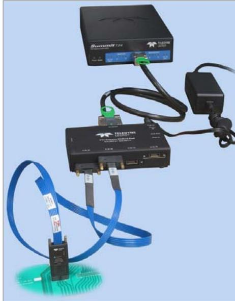
The PCIe 2.0 Mid-bus Probe is shown here with a Summit T24 Analyzer, using a half-width probe head. This configuration can capture traffic at lane widths up to x4.
