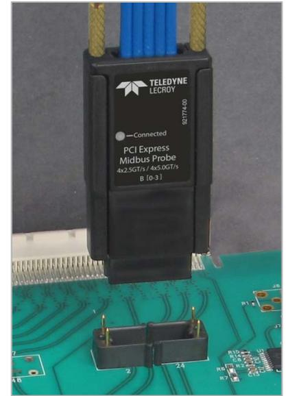
A half-size probe head (shown here) supports up to x4 lane width and attaches to universal 2-piece retention module via thumbscrews.
