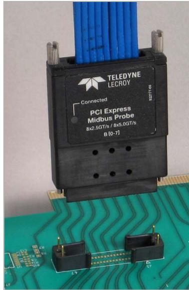
A full-size probe head (shown here) supports up to x8 lane width and attaches to universal 2-piece retention module via thumbscrews.
