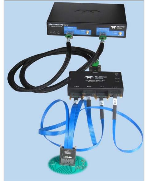
The PCIe 2.0 Mid-bus Probe is shown here with a Summit T28 Analyzer, using a full-width probe head. This configuration can capture traffic at lane widths up to x8. For x16 configurations, use a Summit T3-16 Analyzer (or two Summit T3-8 Analyzers) and two probe pods using full-width probe heads.
