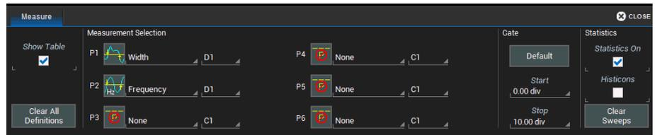
**Figure 1: The Measure Setup showing P1 set for measurement of width and P2 set for measurement of frequency.**
