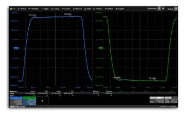
Maximum Transmitter Output Droop — The output droop is calculated on both the "+1" and "-1" symbols in the Test Mode 1 or 6 waveform. The magnitude of the droop is measured with respect to an initial peak value after the zero crossing (Vinit) and the value a defined amount of time after the initial peak value (Vdelay).
