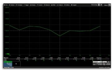
**Transmitter Distortion** — The peak distortion is determined by capturing output from the DUT while it is in Test Mode 4. The MATLAB script provided in the specification removes the disturbing sine wave and measures peak distortion at equally spaced phases of the symbol period. To pass, the script must report less than 15 mV distortion for 10 records.
