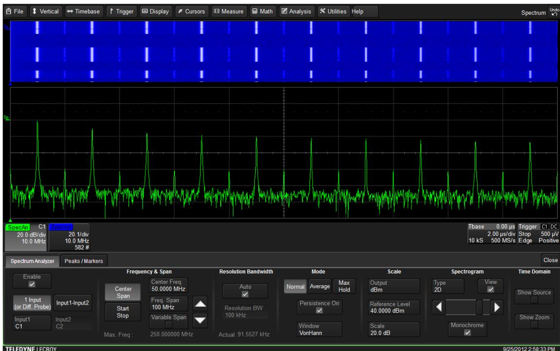
3. Move the Spectrogram **slider** or touch the **Right/Left Arrow** buttons to increase or decrease saturation level.
