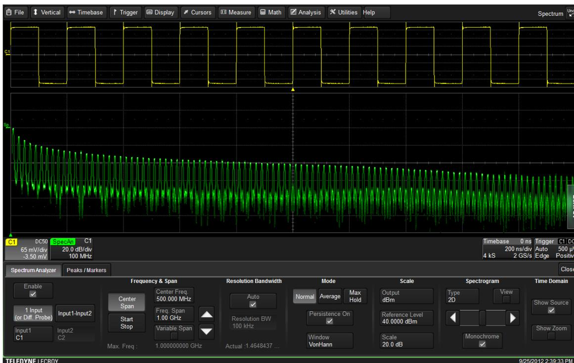
2. To use **1 Input** or a differential probe connected to a single channel (the default), touch **Input1** and choose any channel, zoom, math, or memory source.
