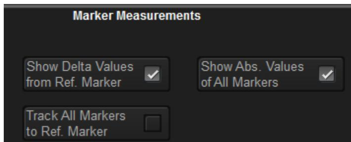
**Note:** The **Track All Markers to Ref. Marker** option locks all markers at their current delta from the Reference Marker. The markers are moved as the Reference Marker is moved. This is useful for finding interesting harmonics in the spectrum.
