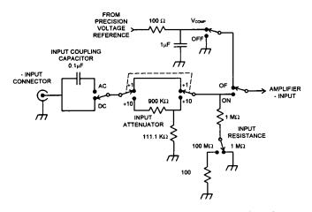
The -input has the same coupling modes as the +input plus one additional option,  $V_{COMP}$  (comparison voltage).
