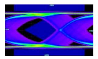
A 2nd-order PLL allows for the user to enter the natural frequency and damping factor to reduce the size of the transition region and to maximize stop band attenuation. Shown here is the same signal with a 2nd-order PLL set to a 1 MHz natural frequency and damping factor of 0.707.
