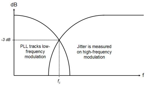
jitter is passed through the software filter, providing for accurate high-frequency jitter measurements.
