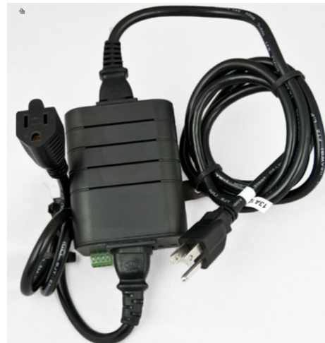
Figure 2: PD Fast Role Swap Compliance Fixture (Note: Fixture includes 110V power cords only)
