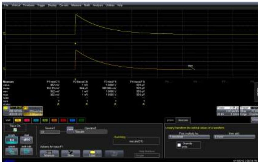
Figure 3: Using the rescale function to normalize the exponential waveform to unity gain
