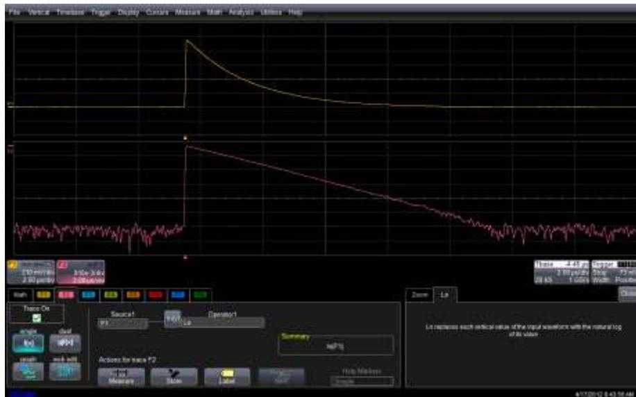
**Figure 5: Using the natural logarithm(Ln) math function to linearize the exponential function. The slope of the linear section of the Ln trace is the reciprocal of the exponential time constant**
