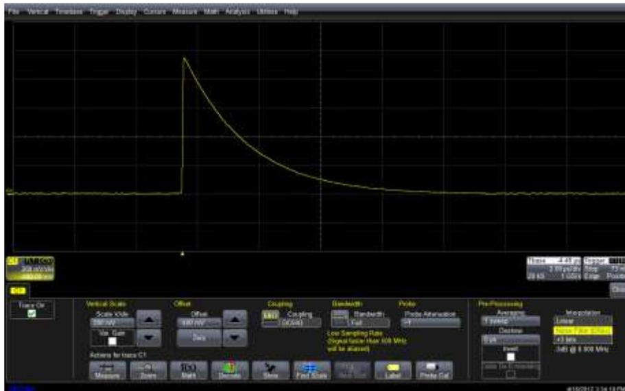
Figure 2: Reducing the noise level on the acquired signal
