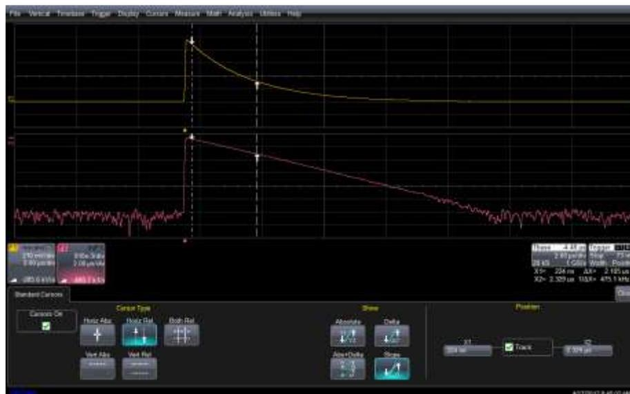
**Figure 6: Measuring the slope of the Ln function to determine the time constant**
