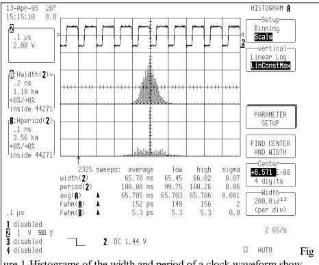
ure 1-Histograms of the width and period of a clock waveform show different distributions of time jitter
