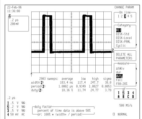
Figure 1 - Direct readout of mean, low/high range, and standard deviation of width, period, and duty cycle measured over 2900 sweeps as shown in a persistence display
