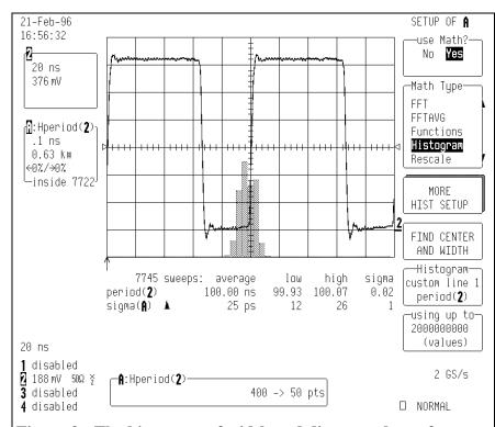
Figure 3 - The histogram of width and direct readout of rms width jitter, sigma(A) and peak to peak jitter, range (A).
