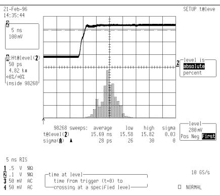
Figure 4 - Time delay of a length of cable used to characterize the jitter due to the oscilloscope.
