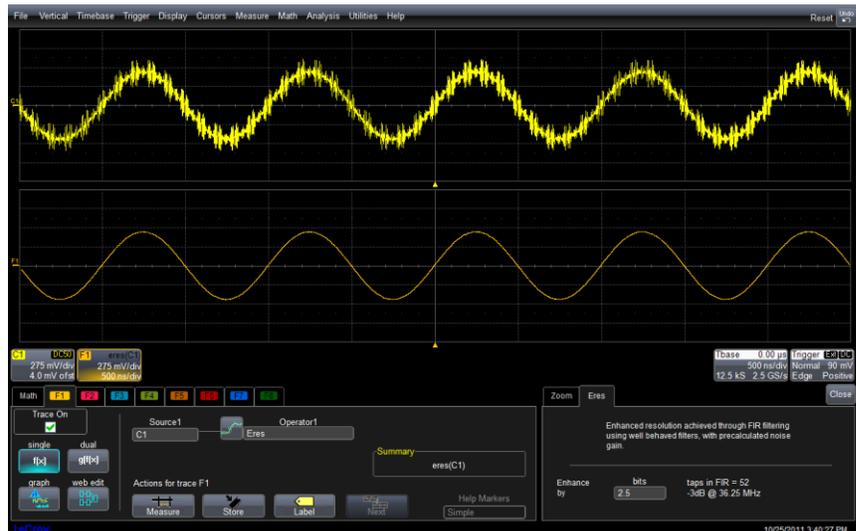
**Figure 1a:** The ERES setup dialog as a math function in the lower right corner. The full bandwidth trace of ADC samples is the upper trace. The lower bandwidth ERES trace is below.
